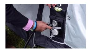
2. Take the awning piping on the cowl and slide it through your awning channel until the awning is in the desired position on the vehicle. (If you are not attaching to a vehicle skip this step).
